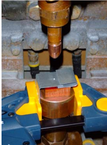
Figure 7: Image showing laboratory setup for indirect hem welding. The hem-inner has been bent to make electrical contact with the lower electrode. The hem-outer is insulated from the lower electrode with a nonconductive material.
